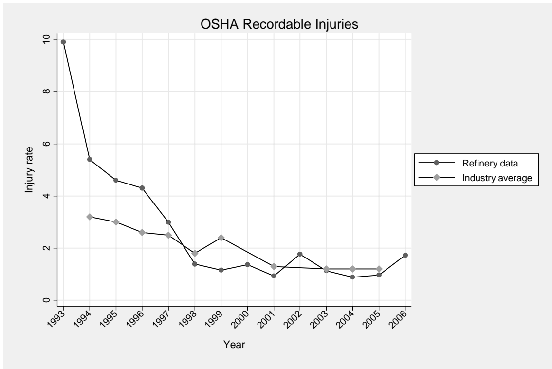
Figure 5 - Safety performance: OSHA Recordable injuries per 100 full-time equivalent workers. Petroleum refining industry average included as benchmark
